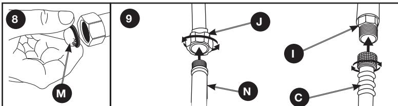
5. Connect water source (N) to pump inlet (J). **NOTE:** Water source must provide a minimum of 5 gallons per minute at 20 PSI.
