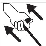
**11****Push the Choke Pin to the OPEN Position**
