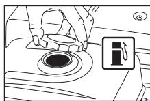
**IMPORTANT:** Ethanol Shield™ (sold separately) is a fuel stabilizer that helps eliminate and prevent ethanol related problems in power equipment. Follow the instructions on the container and add to the gasoline.
