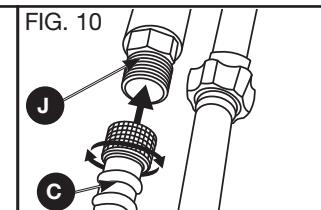
**⚠ WARNING:** To reduce the possibility of contamination always protect against backflow when connected to a potable water system.
