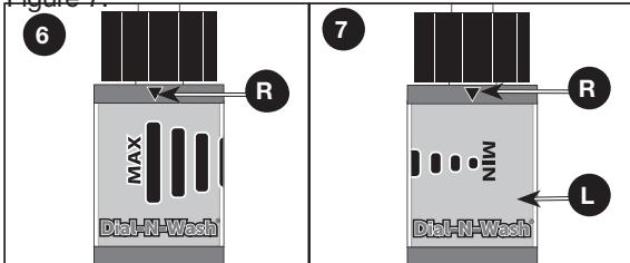
Adjust the pressure by rotating the Dial-N-Wash (L) clockwise for higher pressure or counterclockwise for lower pressure, aligning the arrow with the desired pressure bar on the Dial-N-Wash.
