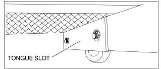
3. Slide lighting wiring through the tongue tube to the front end.
