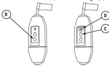
9. Press RESET button (C). The indicator light (D) should be ON.
