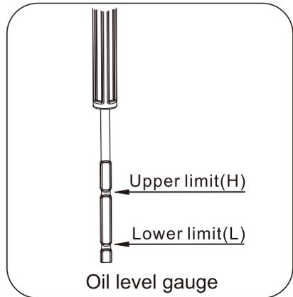
4. Completely insert the dipstick into the dipstick hole during inspection.
