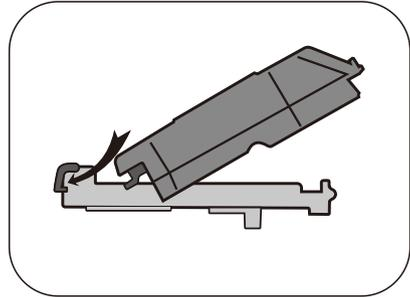
b. Press the cover and secure the retaining clips.
