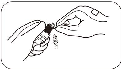
a) Remove the spark plug
