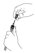
**8.** Select the correct nozzle for your cleaning job per nozzle selection chart in this document and install it onto the lance by pulling the quick-connect coupler back, inserting the nozzle, then releasing the coupler allowing it to snap back in place.
