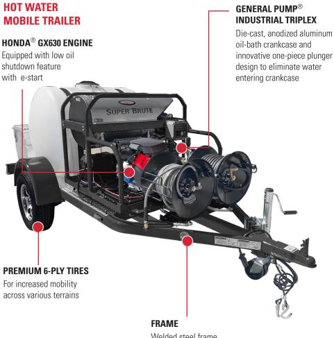
Welded steel frame construction with powdercoated finish for durability and corrosion resistance
