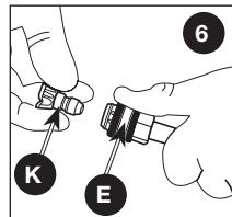
**⚠️ WARNING:** Flying object could cause risk of serious injury. Ensure nozzle is completely inserted in quick-connect socket and quick-connect collar is fully engaged (forward) before squeezing gun trigger.
