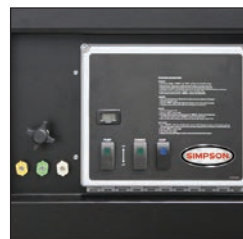
Control panel and on-board nozzles
